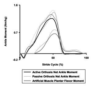
**Figure 2.** Mean + standard deviation of net ankle moments and artificial pneumatic muscle moments for the three subjects during overground walking at 1.0 m/s. Plantar flexion moments are in the positive direction. Subjects walked with very similar net ankle moments for the passive and active orthosis conditions when using foot-swtitch control.
