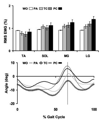
**Figure 5.** TOP: Normalized root mean square EMG of the tibialis anterior (TA), soleus (SOL), medial gastrocnemius (MG), and lateral gastrocnemius (LG) under four conditions: without orthoses (WO), wearing orthoses passively (PA), wearing orthoses under therapist control (TC), and wearing orthoses under patient control (PC). Bars are means  $\pm$  SE. BOTTOM: Mean ankle angle during the gait cycle. Plantar flexion is  $\pm$ .
