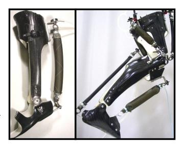
**Figure 1.** ABOVE LEFT: An ankle-foot orthosis with an artificial pneumatic plantar flexor muscle. ABOVE RIGHT: A knee-ankle-foot orthosis with artificial pneumatic muscles providing flexion and extension torque at each joint. Plastic tubes provide compressed air to the artificial muscles from an external air source.
